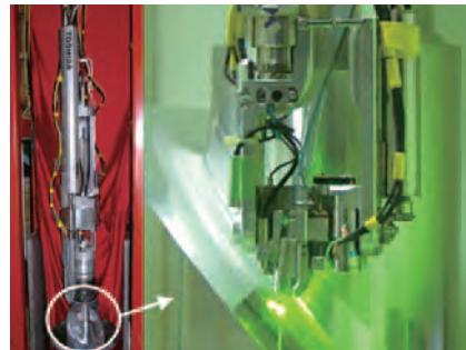
Portable Laser Peening Equipment
